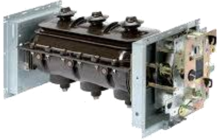
Indoor On-Load switch Rated voltage : 12/24 kV Rated Current : 630A/1250A Rated Short Circuit Current : 16 kA/21 kA Insulation : Sf6
