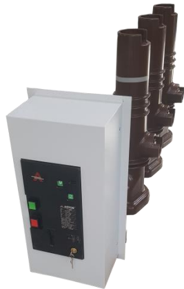
Indoor Sf6 Circuit Breaker Rated voltage : 12/24 /36 kV Rated Current : 630A/1250A Rated Short Circuit Current : 16 kA / 25 kA Insulation : Sf6
