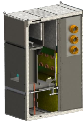
Indoor AIS Metal-Clad Switchgear Rated voltage : 12/24 /36 kV Rated Current : 630A/1250A/2500 A Rated Short Circuit Current : 16/25/31,5 kA Insulation : AIS/Vacuum
