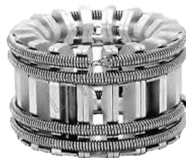
Movable Contact for LBS ( LG ) Rated voltage : 12/24 /36 kV Rated Current : 630A/1250A/ Rated Short Circuit Current : 16/25 kA Insulation : SF6
